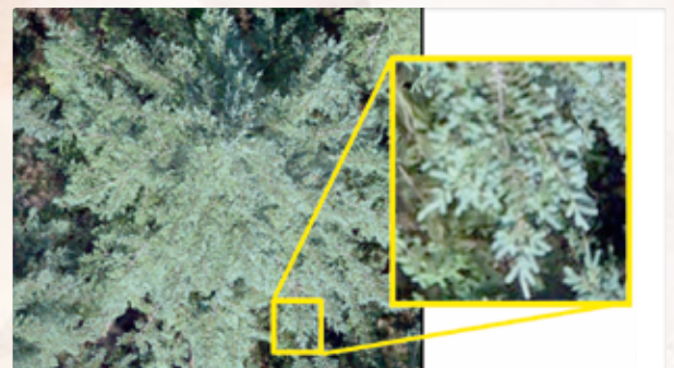
Orthophoto with a ground resolution of 1 cm.
