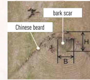
Branch stub buried inside the wood (beech), measuring the height ( H ) and width ( B ) of the bark scar
