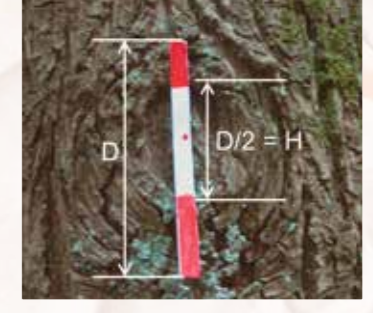
Branch stub buried inside the wood (oak), measuring the size of the bark scar
